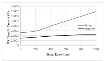
Figure 11 RMS Supply Current vs. Signaling Rate
