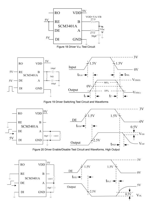
Figure 21 Driver Enable/Disable Test Circuit and Waveforms, Low Output
