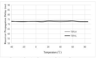
Figure 15 Receiver Propagation Delay vs. Temperature
