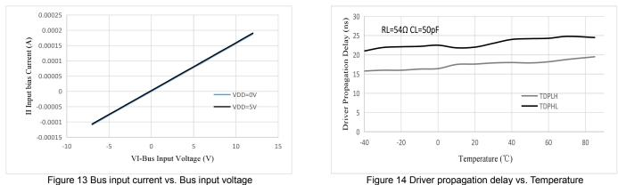
Figure 13 Bus input current vs. Bus input voltage
