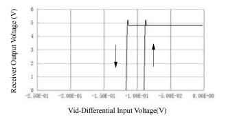
Figure 12 Receiver output voltage vs. Differential input voltage
