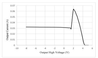
Figure 8 Output current vs. Transmitter output high voltage
