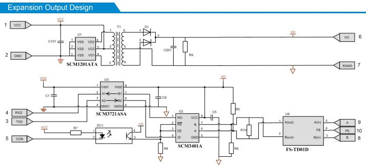
Fig. 26 Schematic diagram of isolation application circuit for UART to RS485 signal
