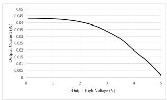
Figure 2 Output Current vs. Receiver Output High Voltage
