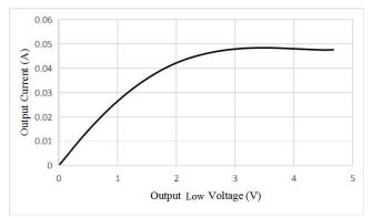
Figure 3 Output Current vs. Receiver Output Low Voltage
