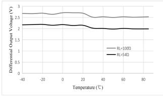
Figure 7 Driver Differential Output Voltage vs Temperature
