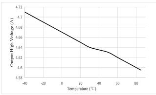
Figure 4 Receiver Output High Voltage vs. Temperature
