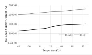
Figure 1 No-Load Supply Current vs. Temperature
