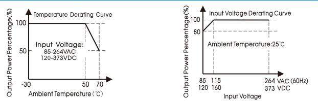
Note: ①With an input voltage between 85-115VAC and a DC input between 120-160VDC the output power must be derated as per the temperature derating curves;
