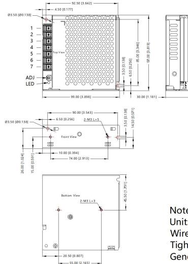
**Pin-Out** Pin Function 1 AC(L) 2 AC(N) 1 3 4 Vo<sub>3</sub> 5 Vo<sub>2</sub> COM 6 7 Vo1
