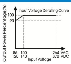
Note: 1. With an AC input voltage between 85 -100VAC and a DC input between 120-140VDC the output power must be derated as per the temperature
