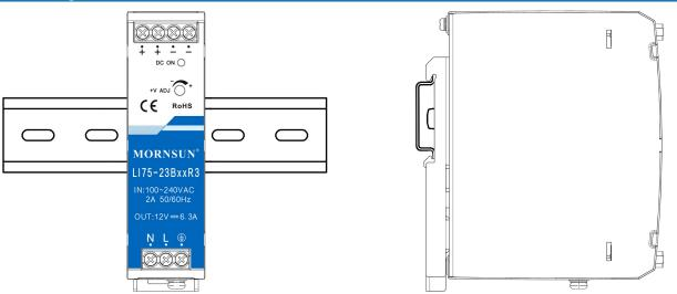
Note: Keep the following installation clearances: 20mm on top, 20mm on the bottom, 5mm on the left and right sides are recommended when the device is loaded permanently with more than 50% of the rated power. Increase this clearance to 15mm in case the adjacent device is a heat source (e.g. another power supply).
