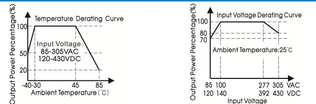
Note: 1. With an AC input voltage between 85 - 100VAC/277 - 305VAC and a DC input between 120 - 140VDC/392 - 430VDC the output power must be derated as per the temperature derating curves;
