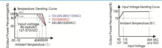
Note: 1.With an AC input voltage between 90 -115VAC and a DC input between 127-162VDC the output power must be derated as per the temperature derating curves;
